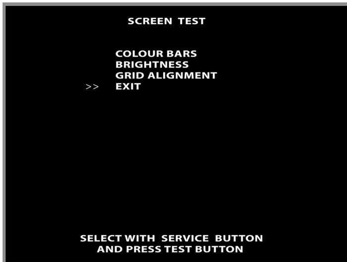
Use the SERVICE Button to move the cursor to the desired test item.
