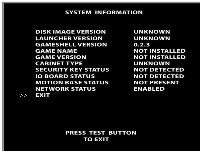
This test displays GENERAL SYSTEM INFORMATION regarding the Hardware Configuration and Software Installed
