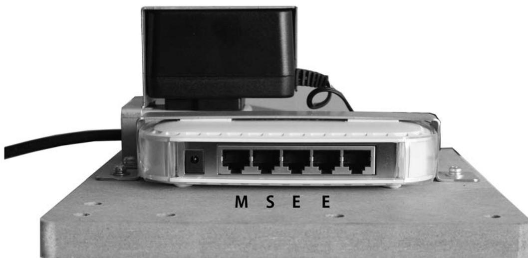
**M = Serial Connection to this Machine's Master Cockpit**
